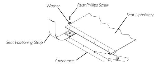
FIGURE 8.4 Replacing Seat Positioning Strap
